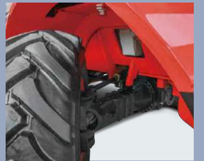
Oscillating steer axle allows either wheel to step over obstacles keeping the truck and load level
